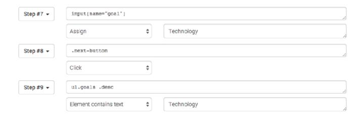
Ghost Inspector is embracing concepts like reusability to help you get more mileage out of your tests. Tests can be nested within other tests as subroutines, so that specific actions can be segmented out and reused. For instance, you can create a "Login Operations" test that logs into your system, and then insert it as the first step of various other tests in the suite. This keeps your login code in one place and makes it easy to maintain if changes to your application occur.
